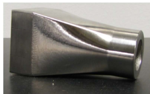
Fig. 7 A PCHE header of alloy 800 HT construction
