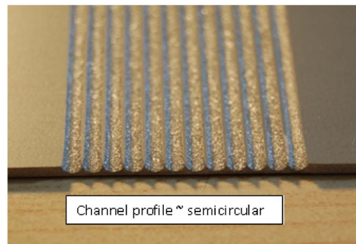
Fig. 6 PCHE channel profile (close to semicircular)
